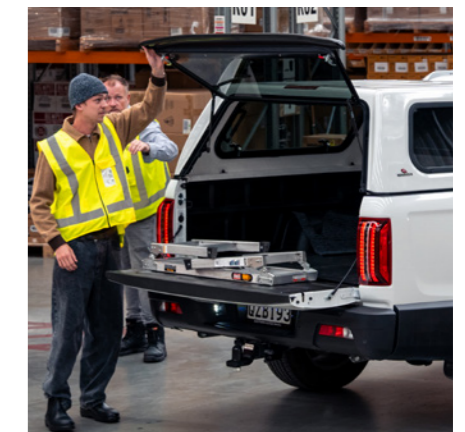
The fibreglass shell eliminates the need for internal framing, maximising useable space.
